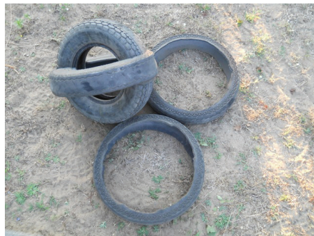
Top: Step 2, notch cut in one tire. Bottom: Step 3, sidewalls cut off two tires, ready to push onto the others.
